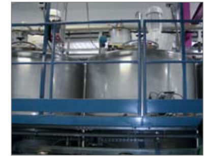
Battery of agitators for dyestuffs with added drying agents.
