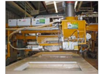
Semi-automatic mortar spraying and extractor system for high-quality serial production of walls. Photo: WeberHaus
