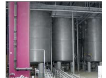
Large agitator tanks used for paint manufacture.
