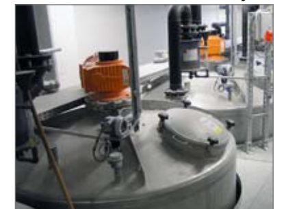
Battery of agitators for viscous material in the chemical industry.
