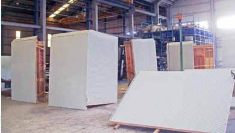
Prefabricated corners for a tank relining.
