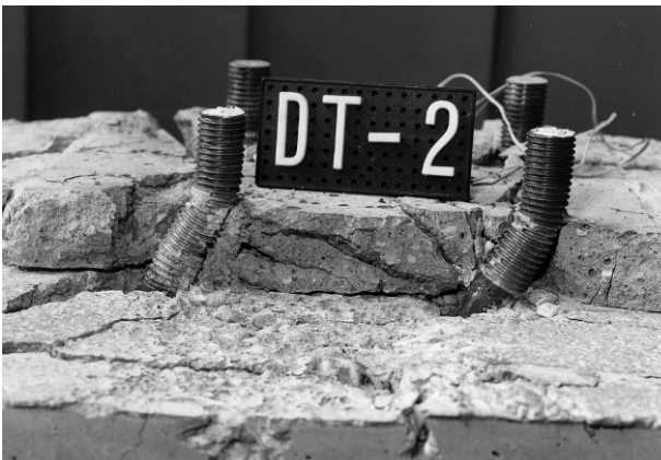
Figure 3: Test specimen loaded by shear force and tensile force (Stevin, 1989)
